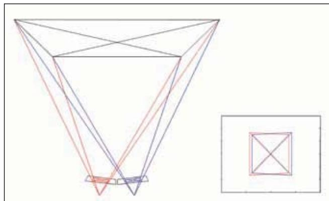
**Figure 5.** Vertical parallax introduced by camera convergence.
