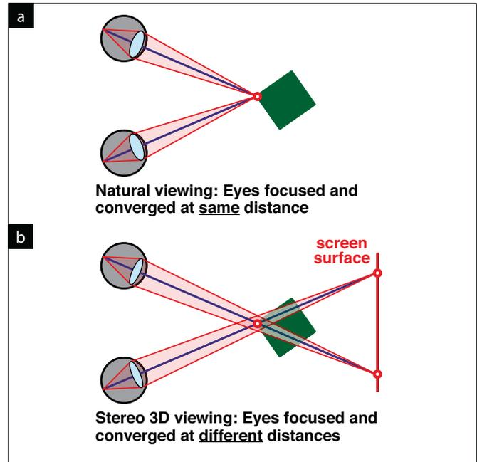
**Figure 11.** The vergence–accommodation conflict in stereoscopic displays. (a) In natural viewing, vergence and accommodation are to the same distance. (b) In stereo displays, these two oculomotor responses must be decoupled for the viewer to have clear, single binocular vision.
