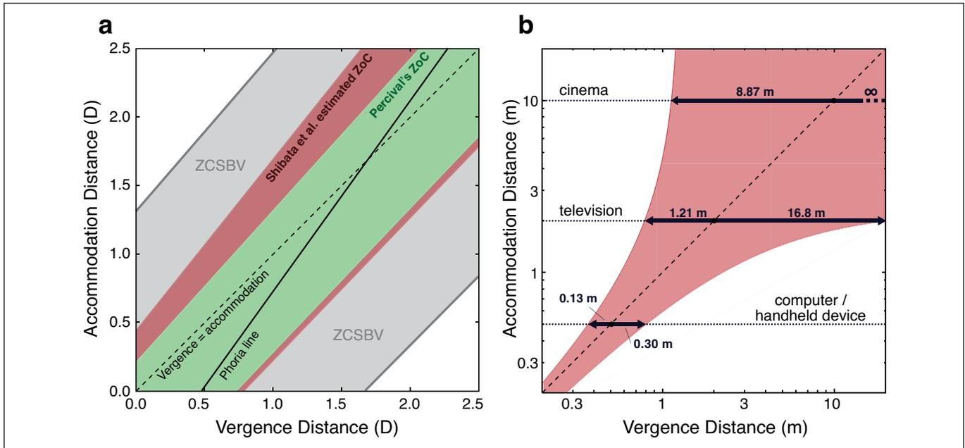
**Figure 12.** ZoC. (a) Plot of accommodation distance as a function of vergence distance, both in diopters. The estimate of the ZCSBV is in gray, Percival's ZoC is in green, and the estimate of the ZoC for S3D viewing from Shibata et al.<sup>64</sup> is in red. The phoria line for a typical viewer is also shown. (b) ZoC from Shibata et al. when plotted in units of distance rather than diopters. The horizontal lines represent the typical viewing distances for various common devices.
