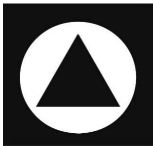
Figure 5. The sticker used as a target for distance tracking. Its dimensions are 37 mm wide by 35 mm high.
